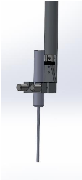
Probe holder with pencil probe
